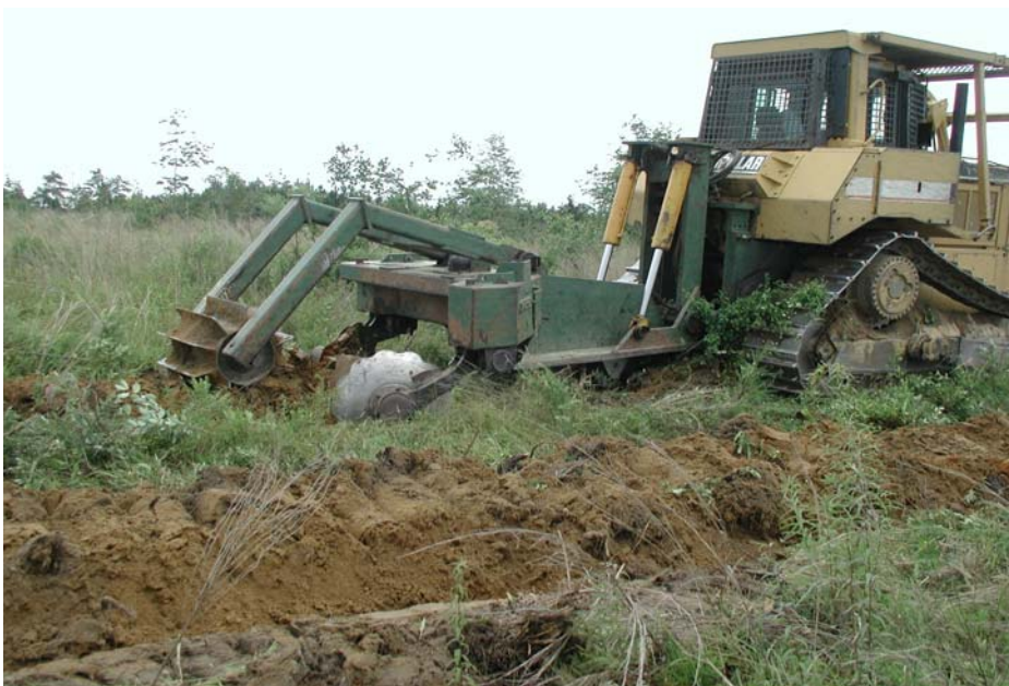
Tractor pulling a combination plow that simultaneously subsoils and beds.
