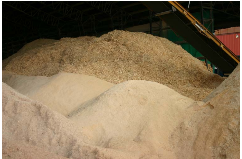
Wood processed to a flour consistency for use in other manufactured materials
